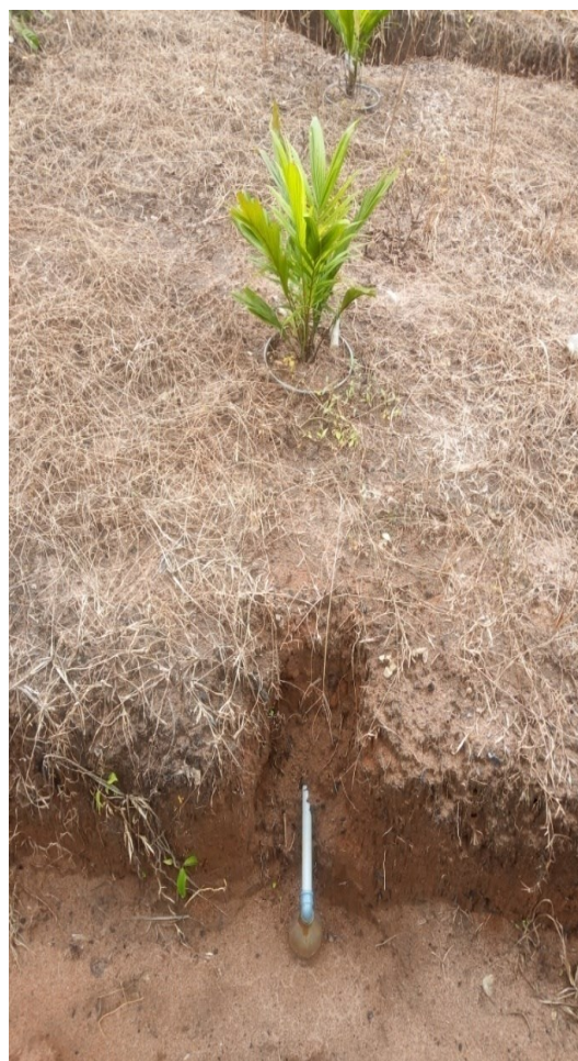
PLATE: 7 A cross section of the Mini-lysimeter showing leachate collection point on the field
