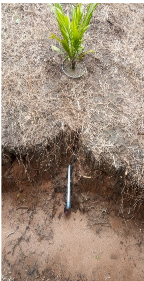
PLATE: 7 A cross section of the Mini-lysimeter showing leachate collection point on the field
